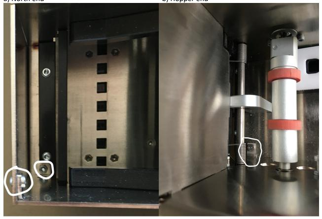
3. Remove the 7 outer screws holding the front panel
