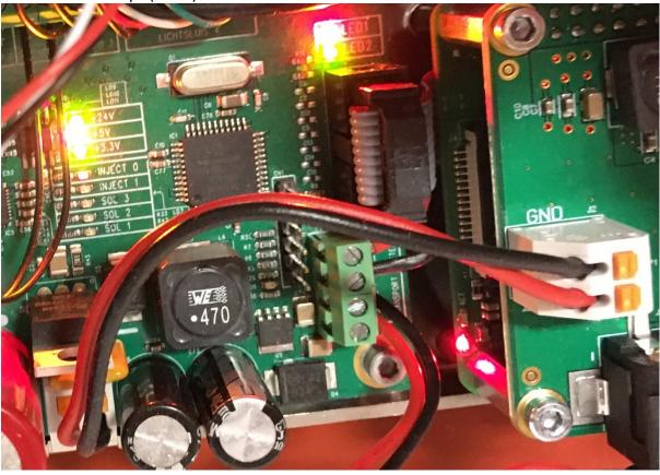
The LEDs marked +3.3, +5V and 24V are self explanatory. LED 1 and 2 giving steady light show that the COM circuits work as they should.
