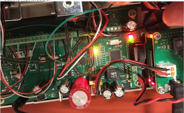
The motherboard gets power from a smaller "in/out" PCB's (white) power cable socket.
