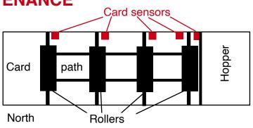
The counters are numbered in the same way as the cards move from the hopper to the slots. i.e. in the cards' direction.
